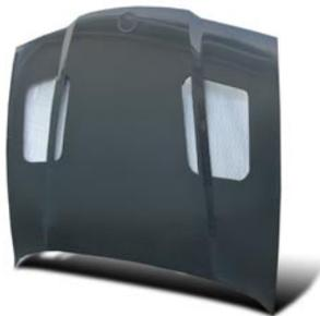
The GTR option is a large scale venting cut out. Includes aluminum grill screens. Compression bonded edges with a special urethane core construction for light rigid parts. Factory style liners, with hardened steel threaded inserts for attaching hinges and latches.
