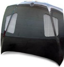
The GTR option is a large scale venting cut out. Includes aluminum grill screens. Compression bonded edges with a special urethane core construction for light rigid parts. Factory style liners, with hardened steel threaded inserts for attaching hinges and latches.
